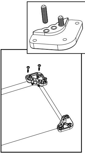
These unique levelers are self-aligning for easy installation. Use the curved tab on the Insert Plate Levelers to locate each Leveler in the corner of the Insert Plate opening and fasten them in to place using three 1-1/4" coarse thread screws per leveler. Be careful not to overtighten.
