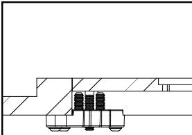
The unique design of the Precision Insert Plate Levelers and adjustable leveling screw system applies pressure to both sides of the insert plate so that – once locked in – your Insert Plate stays flush regardless of the weight applied. The 8 Leveling Screws and 4 Lock-Down screws work together to keep your insert plate flush with the router table surface at all times.
